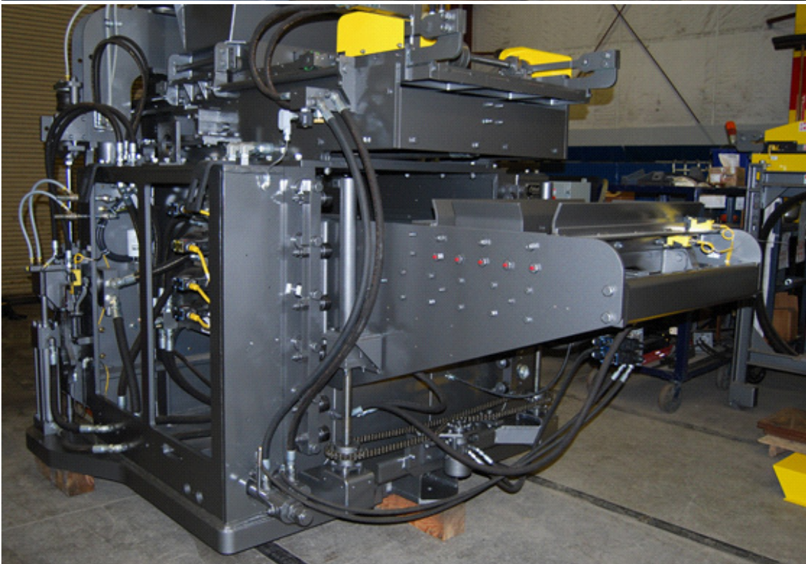
These photos are of a model 1600 block machine at Columbia Machine Inc. being prepped for shipment. Notice the hydraulics located on the opposite side of the pallet feeder.
