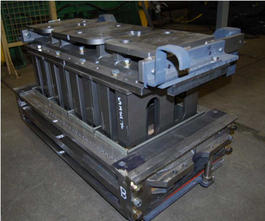
Transit fixture frame with mold (above) and additional transit fixtures shown along with head spacers (below).
